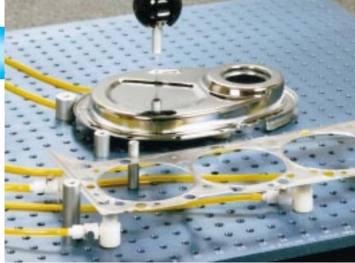
This coordinate measuring system uses OMEGA® couplings to hold complex parts.
